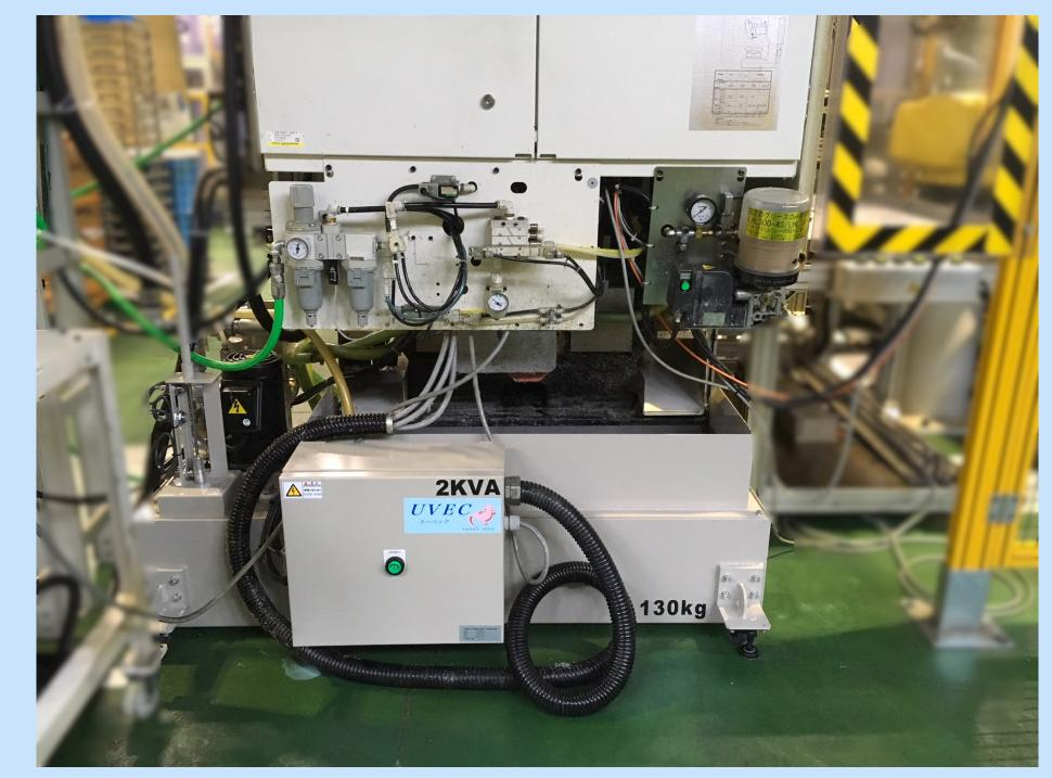
AFTER 回収タンク 切屑はポンプで集中クーラントに返却 Returning the chips to the centralized coolant with a pump in the recovery tank
